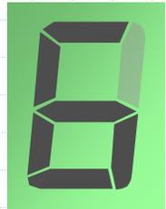
An LCD manufacturer experienced warranty failures where the digits were incorrectly displayed due to missing segments. Failures started to occur after 3 months operation, and were very expensive to repair.
