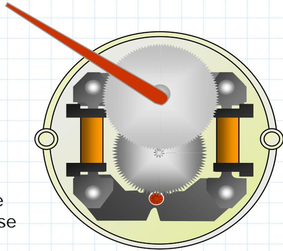
Stepper motors costing less than €1 were causing warranty repairs of €1000 because the indicator would stick.
